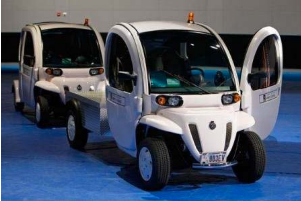
Fig. 2.3 Polaris Industries Neighborhood Electric Vehicles NEVs and Ranger leisure truck with lead acid batteries
