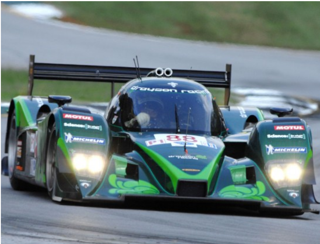
Fig. 3.5 Drayson electric racing car in the UK pioneers many new technologies including continuous charging and structural batteries.
