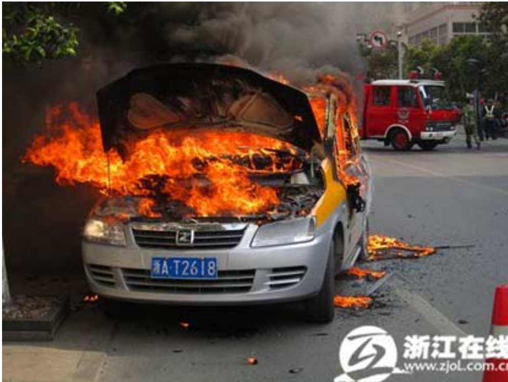
Fig. 2.1 Chinese pure electric taxi with one of the “safer” lithium iron phosphate traction batteries made in China
