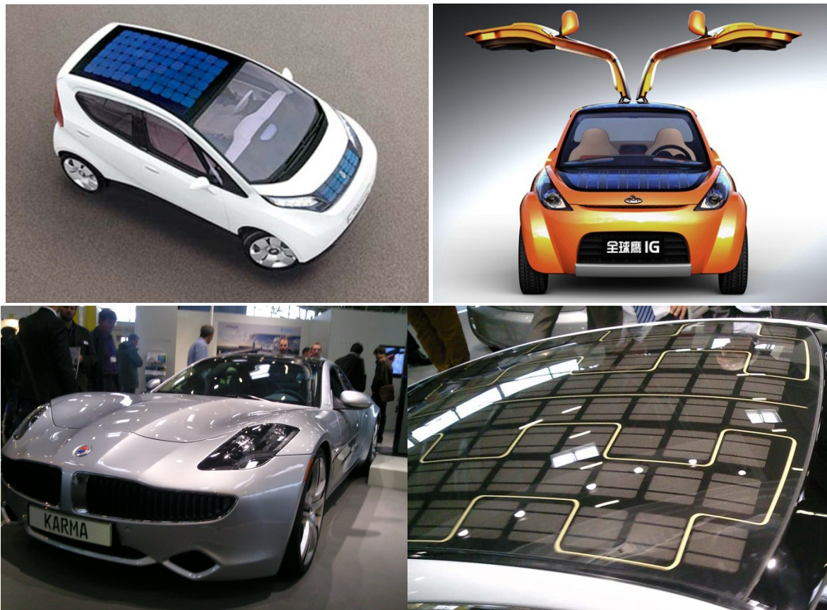
Fig. 3.4 Cars with photovoltaic harvesting. Top pure electric, bottom the hybrid Fisker Karma car.
