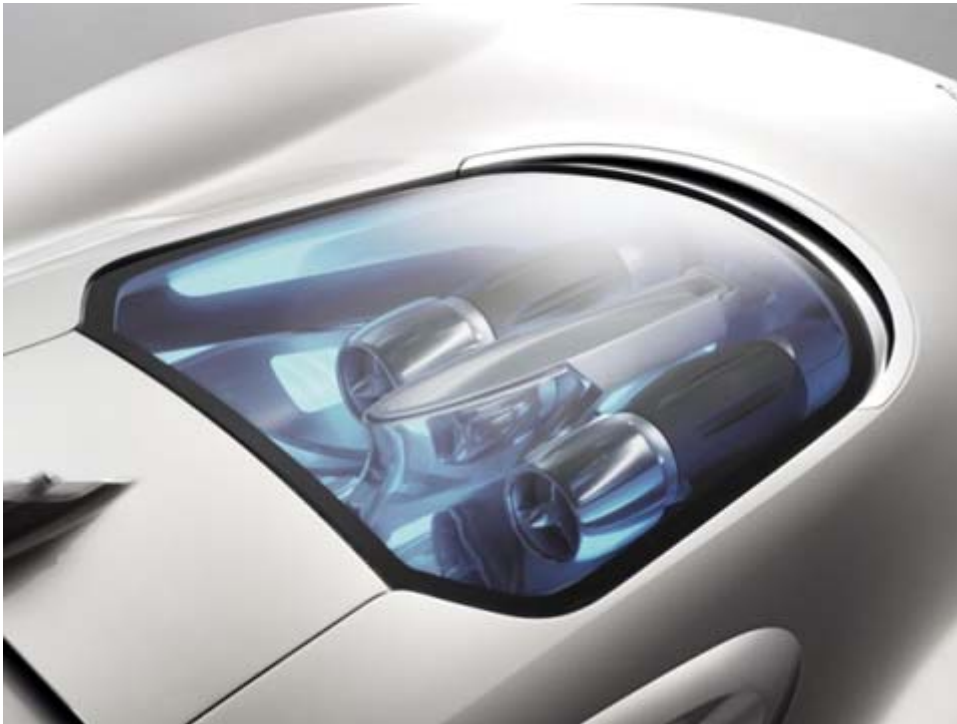
Fig. 3.1 Planned Jaguar long range supercar with two micro turbine range extenders generating 140kW total
